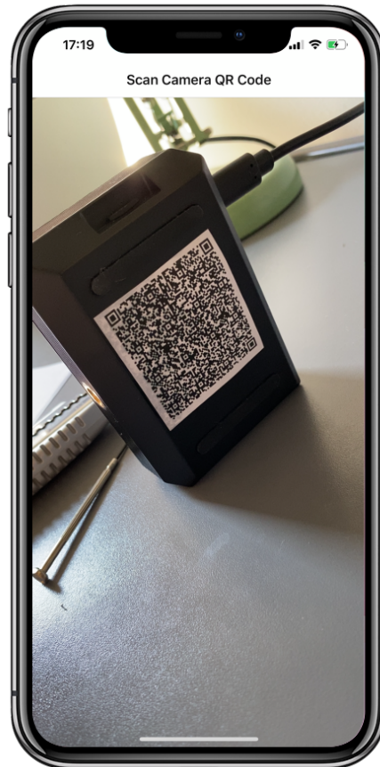
Figure 18: QR code scanner screen, with the viewfinder pointed at the QR code mounted on the camera's case
