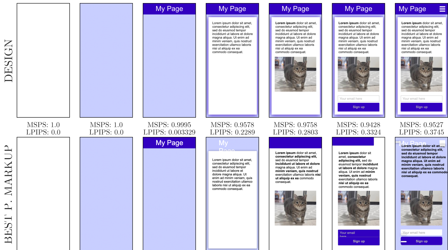
Figure 7.8: The best model output by LPIPS out of 50 samples for each design step, with accuracy metrics between the original design and the resulting web page screen capture. Here, generating svg elements was forbidden, and a lower temperature of 0.5 was used.
